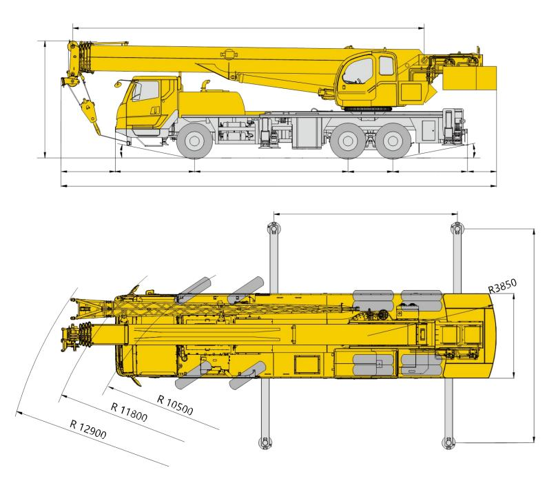
**Note:** When the Qixing cab is configured, the forward extension is 1611mm and the front suspension is 2389mm; when the Xugong car cab is configured, the forward extension is 1624mm and the front suspension is 2376mm.
